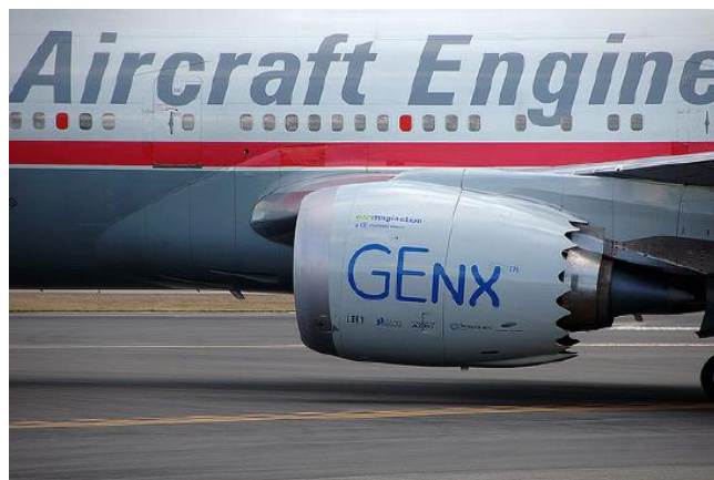
Figure 13.2.3: GE's GENx aircraft engines were developed to meet air travel and cargo companies' needs for better fuel efficiency and faster flights. GE works together with Boeing to integrate the new engines into 747s. Andrew W. Sieber – General Electric – CC BY-NC 2.0.
