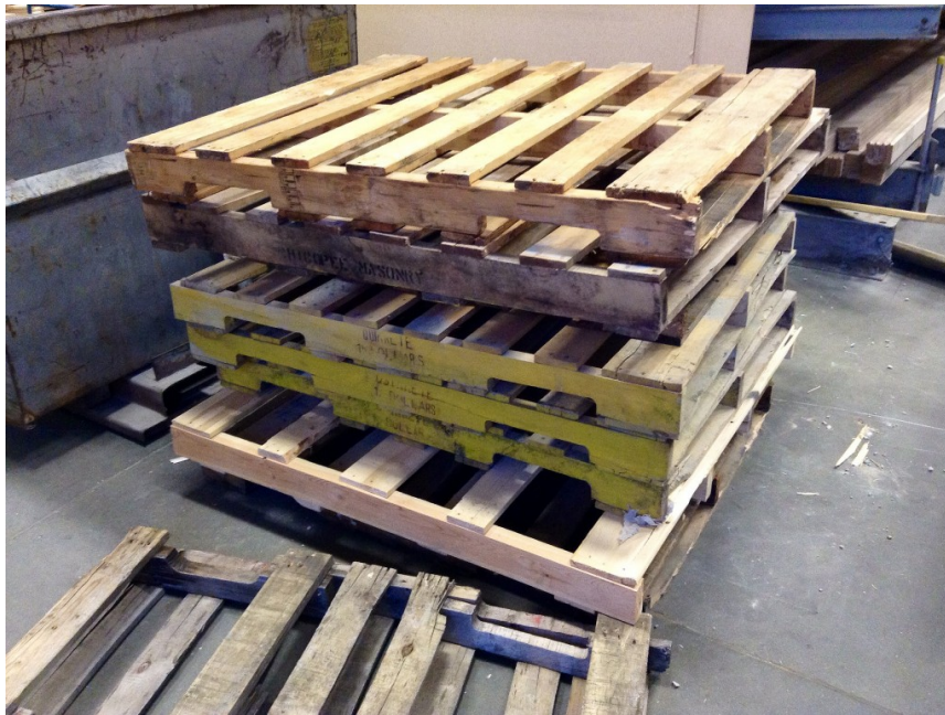
Figure 6.17: This product is bound in tertiary packaging so that mass quantities of it can be stacked on pallets and moved with a forklift. (CC BY 2.0; Mike Mozart via PFlickr )
